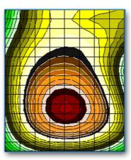
Measurement of the intrusion resistance with Proctornadel. The low intrusion resistance around the medium laid can be clearly seen.
